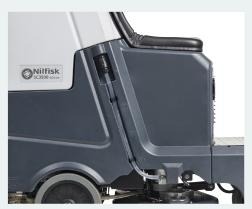
Simple visual monitoring of tank's water level
